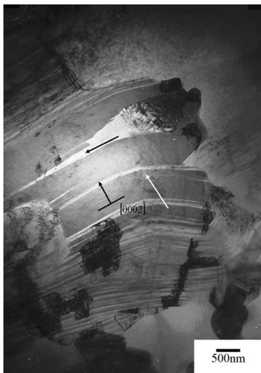
Fig. 4 Bright field image of extruded MgY 3 Zn 1.5 showing the LPSO phase delaminated
